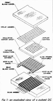
Fig 1: an exploded view of a pulsed DC gas discharge display panel showing the organisation of electrodes and display cavities.
